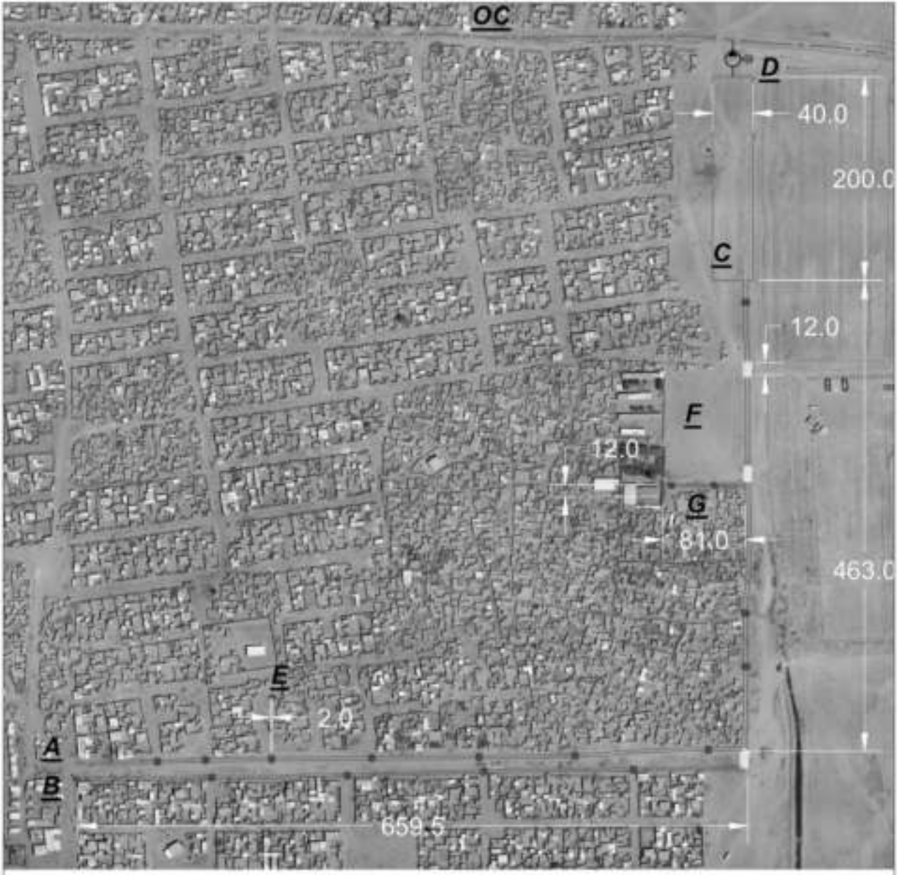
Figure 17, overall view of the proposed intervention. In red are represented the channels (A, B, C, D), dashed red line for the existing channel OC, outlet of collected water; white boxes are the 4 culverts for vehicle transit; in blue the 15 culverts for pedestrian transit. E identify the retention pond. Channel A and Channel B convey water in channel C. Channel C receives also water from channel D and bring water to the retention pond E. Then, collected water is disposed in the existing channel OC using a hydraulic pump (F). P1 to P4 are the relevant points reported in the longitudinal profile of Figure 18
