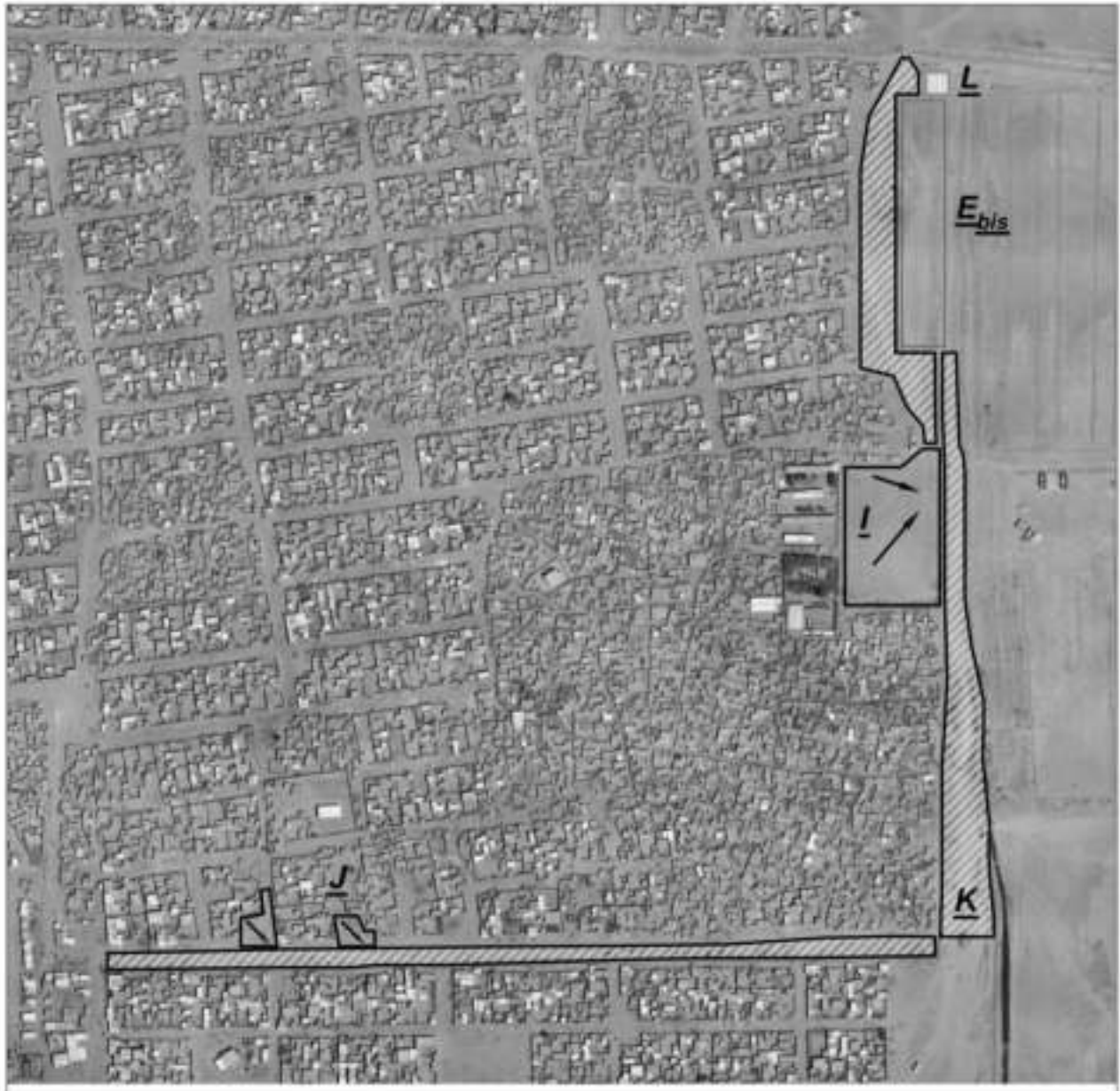
Figure 21, overall view of the proposed reshaping intervention: (I) Emergency paediatric clinic square; (J) internal ponding-prone roads/square; (K) reshaping of traffic roads on the side of the new channels and (L) an elevated platform for pump positioning. Furthermore, (Ebis) indicates the fence needed to protect access to pond (E)
