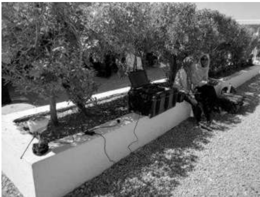
Figure 2: Ground station and GNSS RTK base station (15° 28' 09.1574" lat N, 32° 32' 51.7217" lon E, elevation - ellipsoid 393.180 m - base height: 0.095 m).
